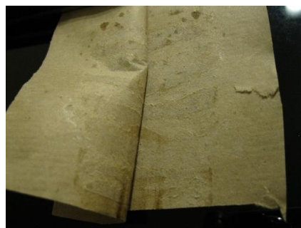
Figure 4.57 Step (vii) of peeling strength test, exhibiting mostly a structural type of failure of the adhesive joint
